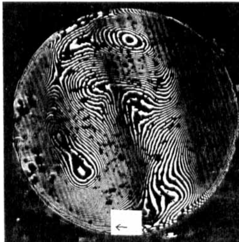
FIGURE 3 Same as Figure 2 but for an FM73M adhesive joint after 144 hours immersion.
